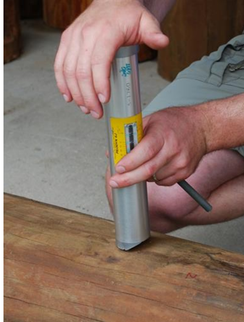
Figure 3. Pilodyn hardness testing.
